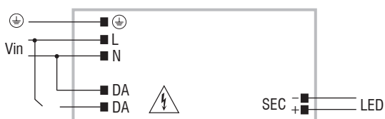
PUSH SWITCH diagram Collegamento PUSH SWITCH
